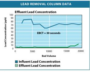
Lead removal by LEI adsorbent in column test; 30 seconds EBCT.
