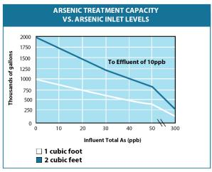
Treatment capacity as a function of tank size.
