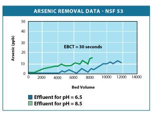
Testing was done under the conditions specified by the NSF Standard 53 for Arsenic. Results at a pH of 6.5 and a pH pf 8.5 are shown in the graph above.
