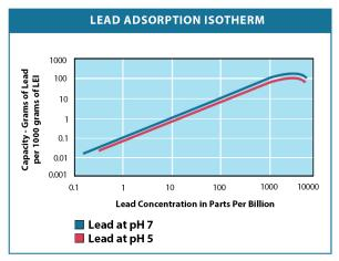
Adsorption isotherms for lead between pH 5 and 7 are nearly identical.
