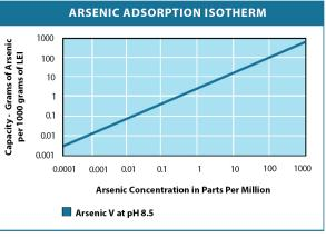
The above graph shows the adsorption isotherm for Arsenic V at pH 8.5.
