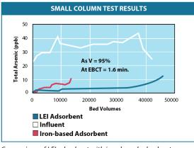
Comparison of LEI adsorbent with iron-based adsorbent.
