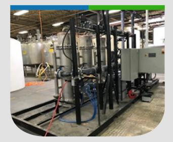
The EF Microfilter skid is fully automated with variable speed controls enabling the operator to set processing flow designs at the most efficient treatment capable out of the highly user-friendly filter, with controls made by Allen Bradley and special features only available with the latest micro-processing technology today.
