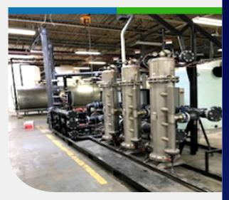
The EF50M4 is built to have the capacity to install 4 microfilter processing stainless steel (SS) filtration units, with a minimum of 20 additional horsepower on the drive pump, larger valving using schedule 80 PVC piping with flow rates up to 15,000bbls/day, doubling the flow of the EF30M skid.
